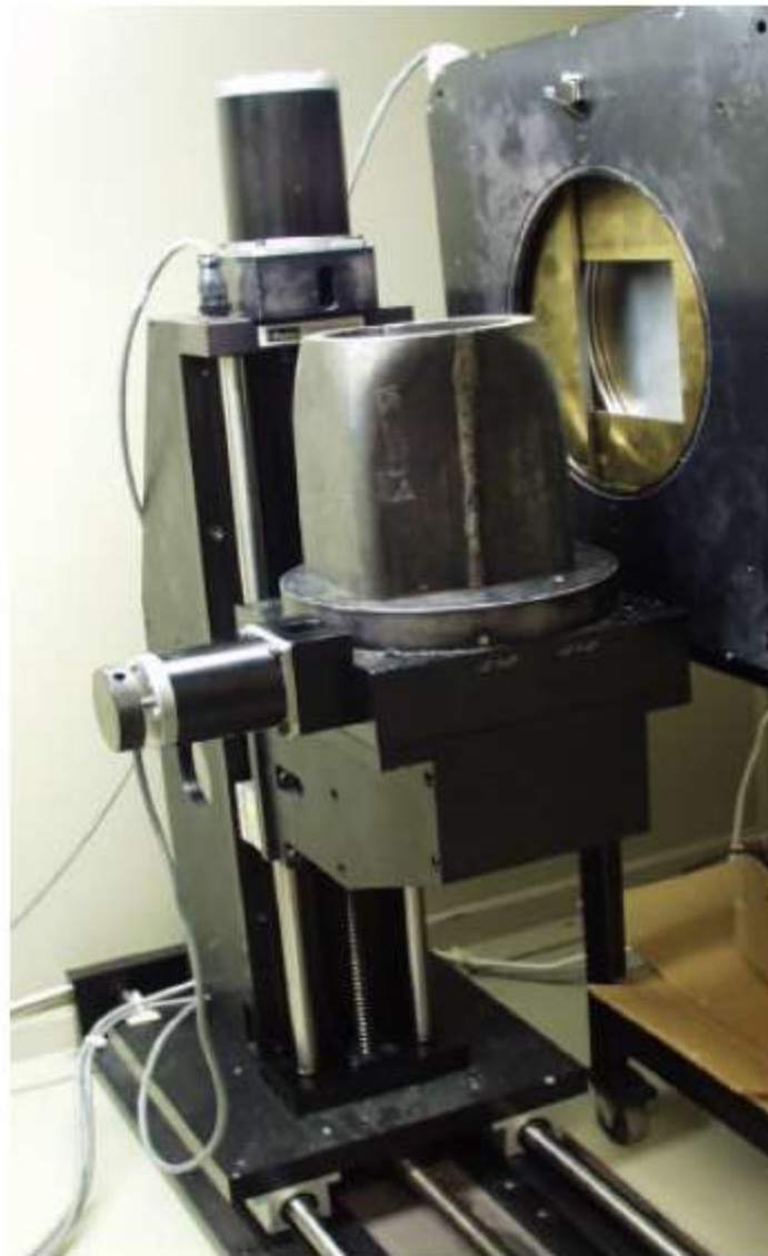
Figure 14. Photograph of a stepper motor controlled sample-positioning system with three degrees of movement.
